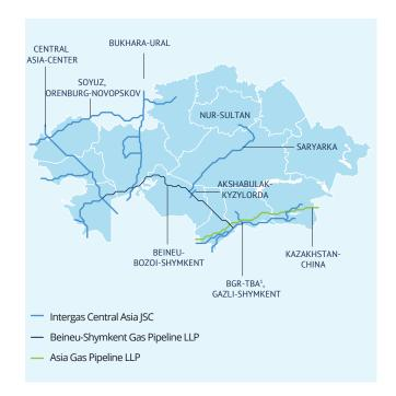
17.85 thous. km total length of trunk gas pipelines
